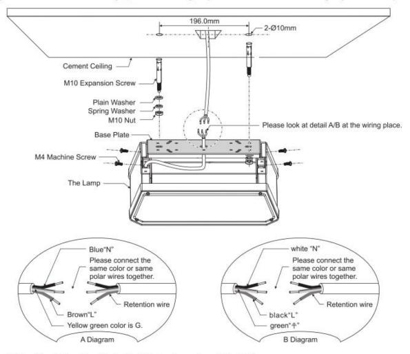
Step one: Drill two holes in the ceiling with electrical drill. Spacing as shown in the sketch.
